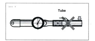
• Only activate the torque wrench at the handle. A marking at the handle shows the position where the force appears.
